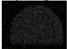
Figure 7, Composition of Sn in reflow bump showing uniform composition.
